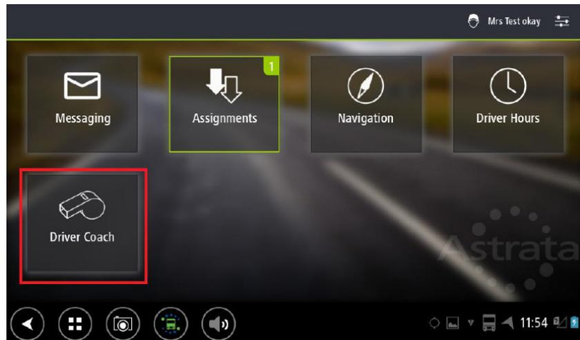
Driver Coach analyses 12 different driving style indicators and communicates a driver's performance compared to his objective in real-time. Soft alerts give gentle reminders about factors like speeding and over-maximum RPM, harsh acceleration and braking, wasted inertia (acceleration quickly followed by braking) and idling
