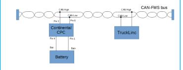
**Note:** The connection of the Astrata OBU to CAN-FMS is a standard procedure, which results in connecting the CAN-High signal to pin 10 of the 18 pin "OBU to truck interface connection", and CAN-Low to pin 11. Below is a description of the E harness and connectors
